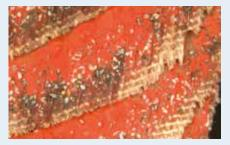
Typical wear pattern with its characteristically shiny cooling film (not glazing!).
