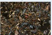
Chips produced with conventional grinding wheels or flap discs. Blue colouration due to overheating.
