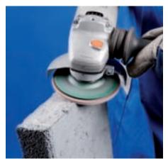
This uncommon flap disc offers a unique solution for applications where surface finish demands are higher than can be achieved by conventional silicon carbide grinding and cup wheels. Designed for grinding on hard to machine metals, plastics and masonry products.
