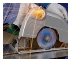
Performance cut-off wheels with diamondshaped bore for use with circular saws. Includes 5/8" and 1/2" adapters for use on angle grinders and straight shaft grinders.
