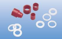
PFERD bench grinder bushings provide a safe method of reducing the wheel arbor to accommodate various spindle sizes. The bushing should be flush on both sides of the wheel, and should not interfere with the flanges.
