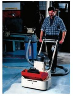
Floor rubs are available in three different grits for rough grinding to smooth finishing on concrete and other masonry surfaces. Silicon carbide rubs are vitrified bonded for wet or dry use. Wooden wedges for mounting rubs are also available.
