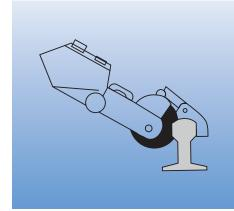
Special-purpose wheel for cutting metal roof and floor decking and rails with portable cut-off machines.
