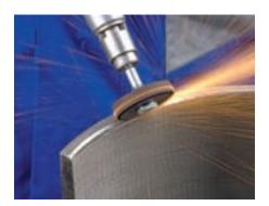
Accessory for mounting snagging wheels on straight grinders.
