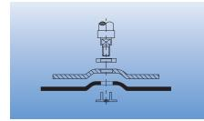
Use the backing pad when mounting SG-FLEX wheels on an angle grinder. Backing pad controls wheel flexibility to provide optimum level of removal and surface finish.
