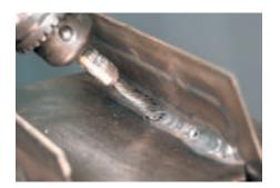
SINGLETWIST<sup>®</sup> end brushes are produced with a single, twisted wire knot, designed especially for brushing internal corners and edges where access is limited. Wire filament is with a left handed twist of the brush rotation, which prevents the knots from unravelling during use.
