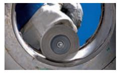
Crimped brushes provide lighter brushing action and superior finish when cleaning, removing rust and paint, smoothing, cleaning cast seams, light deburring.
