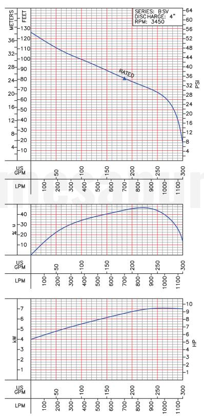
Testing is performed with water specific gravity of 1.0 @ 68 °F (20 °C); other fluids may vary performance.
